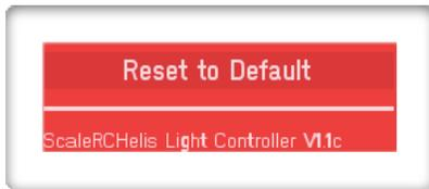
Connect. You may also have to power cycle the controller. This will clear the stored parameters and return the controller back to the default parameters it was shipped with. You will also see your firmware version listed here also.
