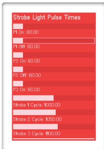
Off Time for the last strobe. The off time is controlled by the Strobe Light Cycle Times. If you do enter a time into the last Strobe Off Time, you will notice a short pulse when there should not be one.
